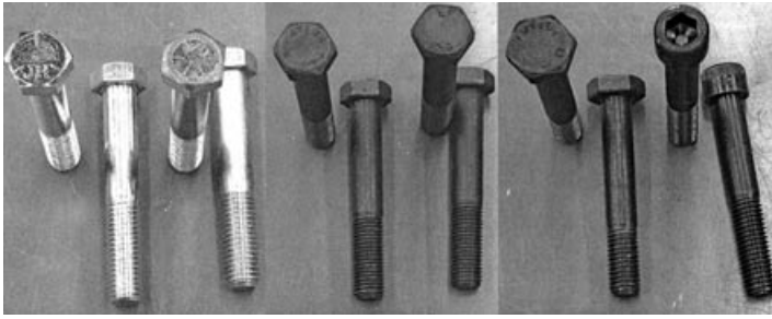
Fig. 1 Selection of bolts illustrative of the ready availability of a variety of technically important, clearly identified materials for testing. From left to right: Grade 5, Grade 8, Metric 8.8, Metric 10.9, A325, A574 socket head.
