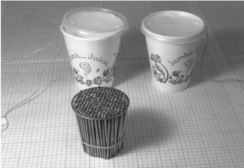
Fig. 2 The Styrofoam cup calorimeter. The cup on the left normally holds the aluminum core that has been removed and placed in front of it. This core is constructed from 184 aluminum rods, 2.38mm in diameter and 60mm long. The rods are held with a circular plate drilled to keep them separated. Water just covers the top of the plate when the core is in the cup. The cup on the right is filled only with water. Both cups have the same height of water and are closed with plastic lids. Each cup is instrumented with two thermocouples, one near the surface of the water and one near the bottom.
